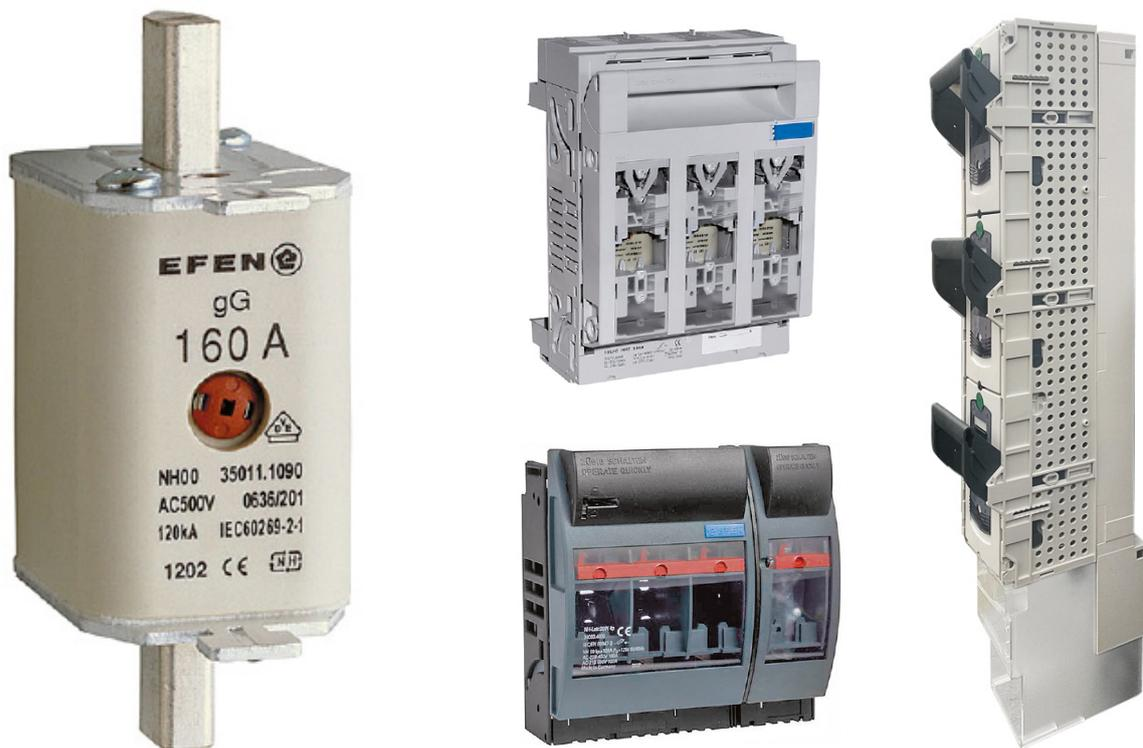
**NH stands for “low voltage high rupturing capacity” (from the German: Niederspannungs Hochleistungs Sicherungen). NH fuses have a breaking capacity generally exceeding 100 kA, which covers virtually all the short-circuit currents expected to be encountered in low voltage systems.**
